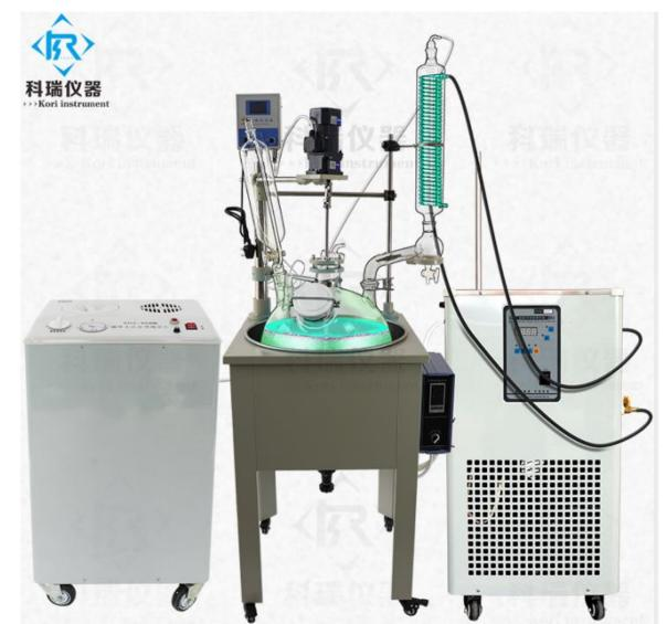
Middle Single layer glass reactor + Water ring vacuum pump + Chiller
